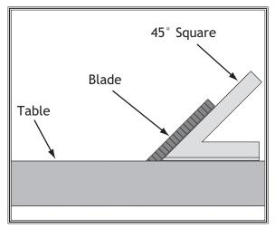
Figure 91. Checking the blade at 45°.
